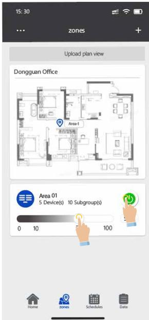
Press the button or slide the bar to quickly on/off or dim the zone devices without entering into the zone.
